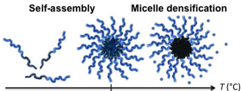
Figure: Diblock elastin-like polypeptides (ELPs) are random-coils at low temperature and spherical aggregates above the critical micelle temperature (CMT), followed by a progressive dehydration of the micelle core.
