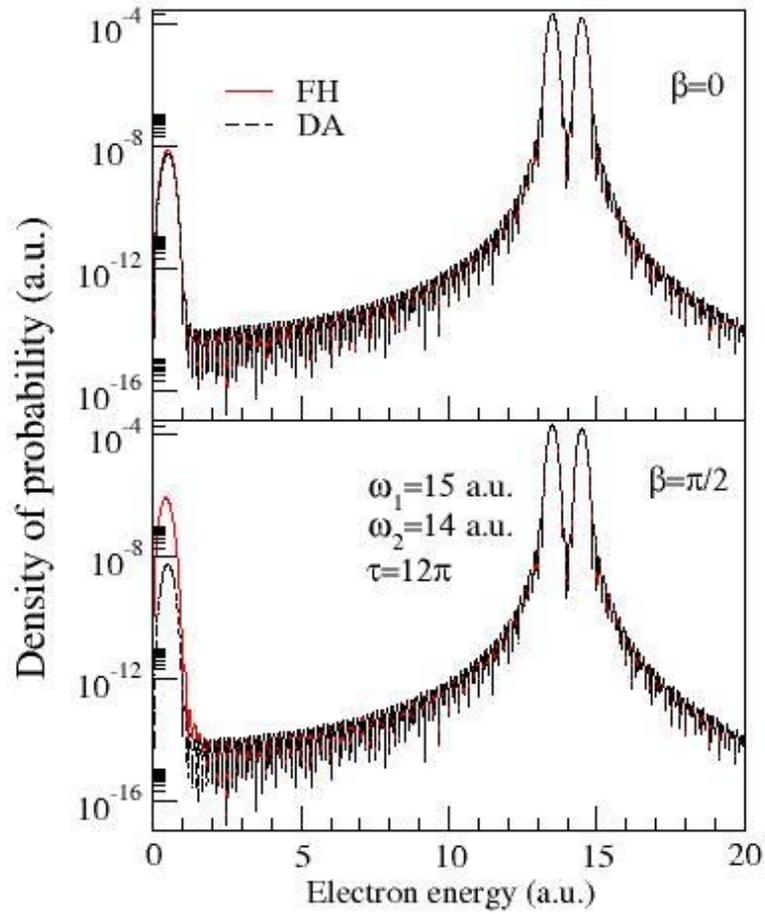
Figure: Photoelectron spectra calculated in nonperturbative approach, solving the TDSE. Calculations are performed using the full Hamiltonian (FH) and in dipole approximation (DA). The laser intensity is  $3.51 \cdot 10^{16} \text{ W/cm}^2$ ,  $\beta$  refers to the relative propagation angle of the two electromagnetic fields (see the text).
