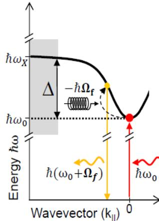
Figure: Principle of polaritonic cooling. The black curve is a typical lower polariton dispersion. The red spot and arrows figure the optically pumped polaritons (of energy  $\hbar\omega_0$ ). Some of the pumped polaritons are scattered by thermal phonons (spring-like arrow) and thus gain an average energy  $\hbar\Omega_f(T)$  (i.e. the average thermal phonons energy) and finally recombine by emitting photons (yellow arrows).
