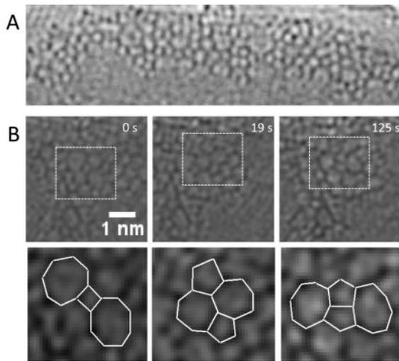
Figure 1: Structural defects in the hexagonal silica network grown at 470°C on a Ru surface. (a) Arrangement of vertical defect lines (pentagon pairs, interrupted by heptagons or octagons) in a partially ordered network. (b) Reconstruction of a typical defect as a function of time.
