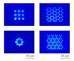
Figure 1: Fluorescence images of single atoms trapped in microtrap arrays with different geometries [4].
