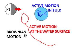
Figure : Trajectories of Janus colloids showing Brownian motion (in absence of  $H_2O_2$ ), and the active motion in bulk and at the air-water interface ([ $H_2O_2$ ]=5%).
