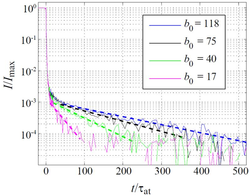
Figure 1: Slow decay of the fluorescence for different on-resonance optical thickness  $b_0$ . The solid lines are experimental data and the dashed lines are exponential fits allowing the measurement of the decay rate.
