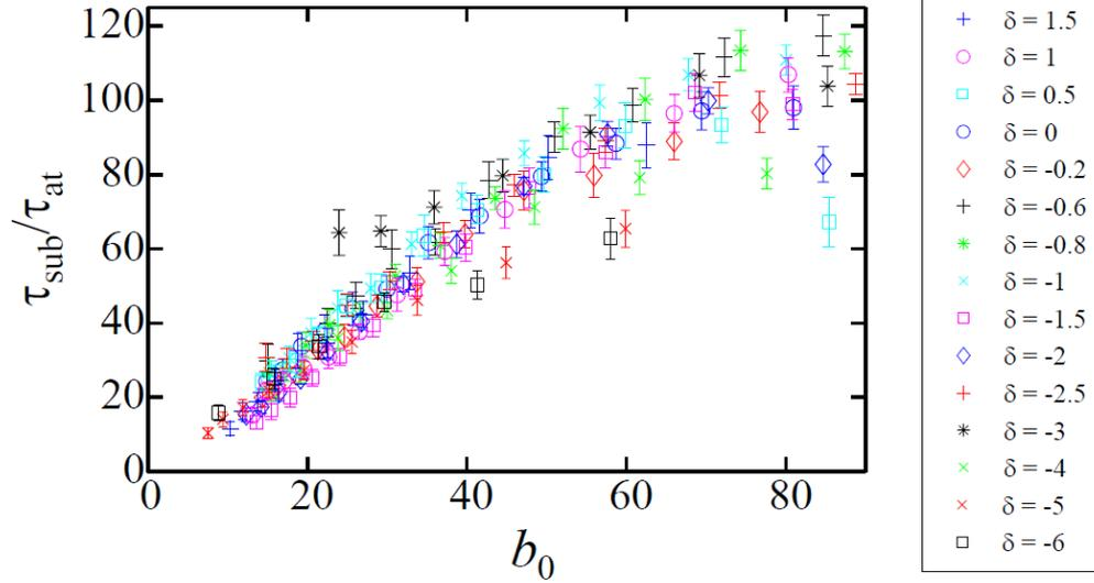
Figure 2: Subradiant time constant  $\tau_{\text{sub}}$  (in unit of  $\tau_{\text{at}}$ ) as a function of the on-resonance optical thickness  $b_0$  for different detunings  $\delta$  (in unit of the natural linewidth  $\Gamma$ ) of the probe laser. Almost all points collapse on the same curve showing the linear scaling of the time constant with the on-resonance optical thickness.
