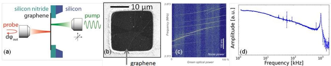
Figure 1: (a) Cavity-free optical pump-probe setup, (b) SEM image of a suspended graphene membrane, (c) Frequency anti-crossing of the coupled resonators, (d) Bode diagram of the response of the graphene resonator to an external drive. It clearly shows the thermal low-pass behaviour and the first mechanical resonance mode
