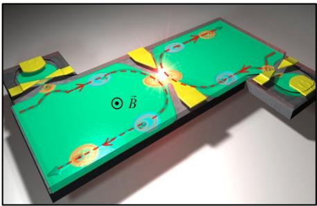
Sketch of electronic Hong-Ou-Mandel experiment: the two dimensional electron gas is pictured in green, the metallic gates in gold and the edge channels by red dashed lines
