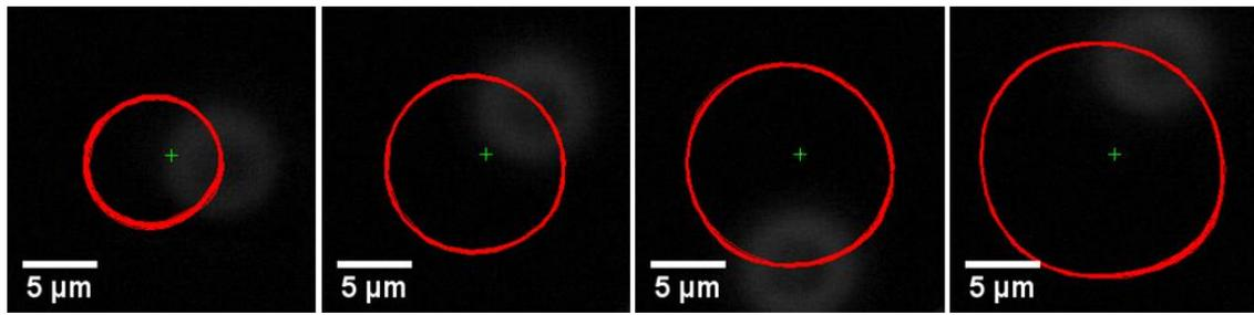
Figure 2: Particle's orbits around the laser beam axis (marked by a blue cross).  $\omega_0 = 4.3 \mu\text{m}$ . The orbit radius increases with the laser power (3.2, 7.0, 10.1, 19.6 mW, from left to right).
