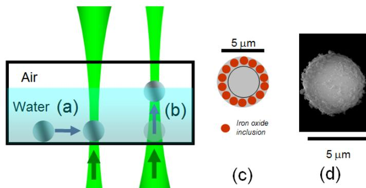
Figure 1: Optical capture (a) and levitation (b) of a particle up to W-A interface. Sketch for the internal structure of a magsphere (c) and electron microscope view of the particle surface (d).
