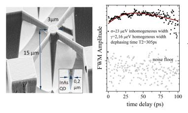
Figure 1: Left: SEM image of a cone shaped GaAs-based photonic trumpet. Such a waveguide, efficiently couples ( $\beta$ -factor around 0.4) the laser pulses with the QDs, located at the tip of the trumpet (inset). Right: Delay dependence of the FWM, yielding homogenous width of  $\gamma = 2.16 \,\mu eV$  in a presence of inhomogenous broadening of  $\sigma = 23 \,\mu eV$ .
