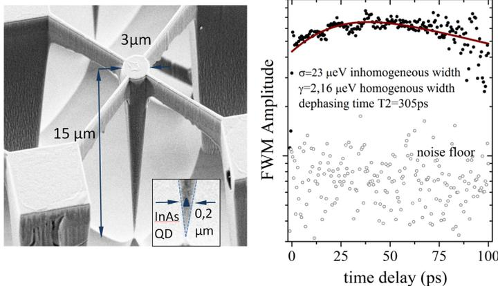
Figure 1: *Left: SEM image of a cone shaped GaAs-based photonic trumpet. Such a waveguide, efficiently couples ( $\beta$ -factor around 0.4) the laser pulses with the QDs, located at the tip of the trumpet (inset). Right: Delay dependence of the FWM, yielding homogeneous width of  $\gamma = 2.16 \mu\text{eV}$  in a presence of inhomogeneous broadening of  $\sigma = 23 \mu\text{eV}$ .*
