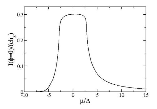
Figure 1: Current *I* vs chemical potential  $\mu$  calculated for a nanowire with a short normal part at small transverse magnetic field  $h_z/\Delta=0.1$ , and at  $\phi=0$ ,  $h_x/\Delta=3$ , and  $m\alpha^2/\Delta=10$ . Here  $\alpha$  is Rashba spin-orbit coupling strength,  $\Delta$  is the magnitude of the induced pairing potential, and *e* and *m* are the effective electron charge and mass.
