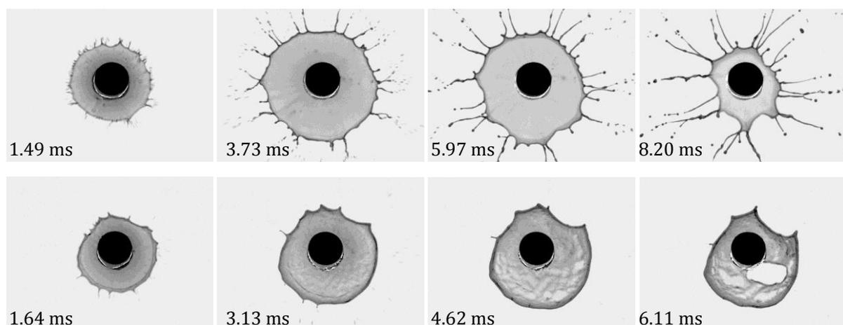
Figure: Time evolution of liquid sheets made of a viscous liquid (top) and of a viscoelastic fluid (bottom). The times indicated correspond to the time elapsed since the drop has impacted the target (shown as the black disk, diameter 6 mm)
