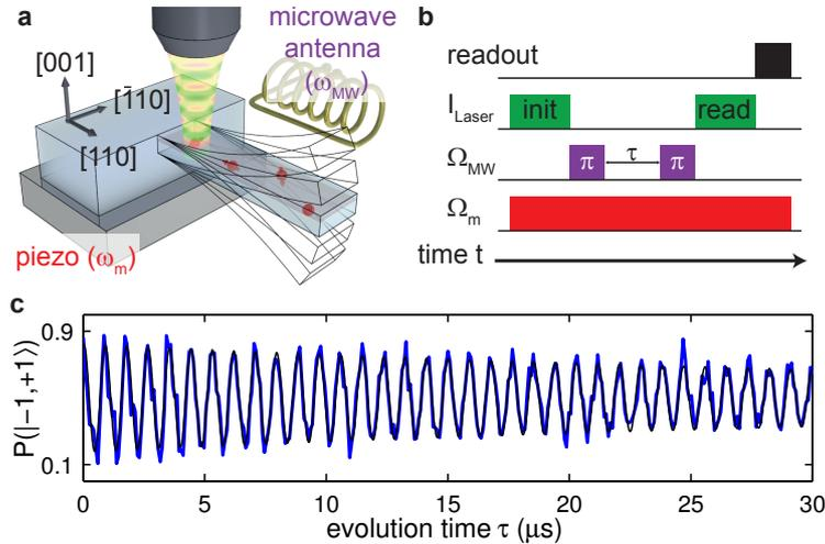
Figure 1: a) Schematic of the system: A Nitrogen-Vacancy defect is embedded inside a single-crystal-diamond mechanical resonator. The microwave antenna and the confocal microscope are used to initialize and readout the spin states. Piezoelectric actuation generates the phononic field. b) Sequence used to generate the strain-driven Rabi oscillations. c) Coherent strain driving of a dipole forbidden transition. Decay time of the Rabi oscillation is around 40  $\mu\text{s}$  at room temperature.
