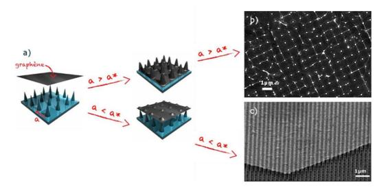
Figure 1: Principle of strain distribution on graphene transferred onto a corrugated substrate: a) sparse silica pillars induce self-organization of ripple formation in domains, b) dense pillar array leads to fully suspended graphene monolayer at the macroscale.
