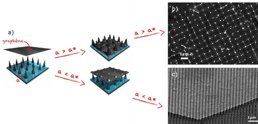
Figure 1: Principle of strain distribution on graphene transferred onto a corrugated substrate: a) sparse silica pillars induce self-organization of ripple formation in domains, b) dense pillar array leads to fully suspended graphene monolayer at the macroscale.
