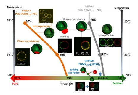
We have clearly shown that the architecture and molar mass of the hydrophobic block have a strong influence on the phase diagram and membrane structuration. When hydrophobic mismatch is expected to be weak, (e.g  $PEO_{400}$ -*b*-PDMS<sub>1500</sub>-*b*-PEO<sub>400</sub>) heterogeneous hybrid vesicles can be observed once the lipid content is above 16% in weight, whereas 50% at least, are necessary with thicker block (PEO<sub>600</sub>-*b*-PDMS<sub>3000</sub>-*b*-PEO<sub>600</sub>).
