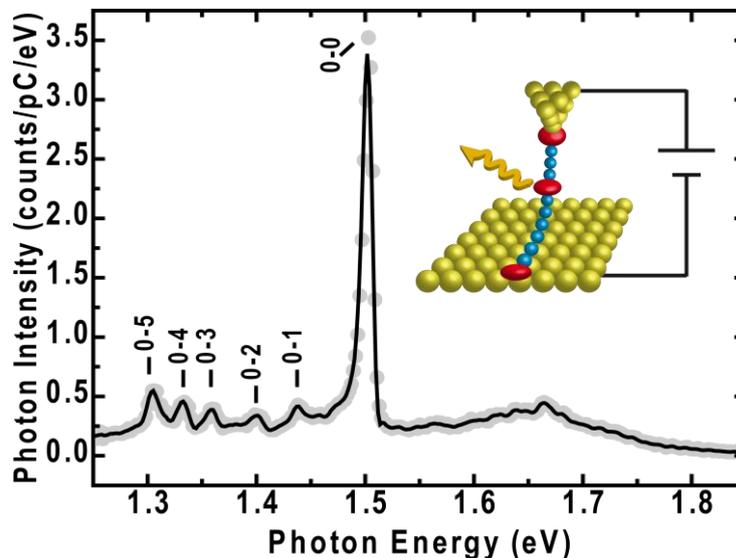
Figure 1 : Characteristic light emission spectra of a suspended molecular wire. In the inset: scheme of the experimental concept.
