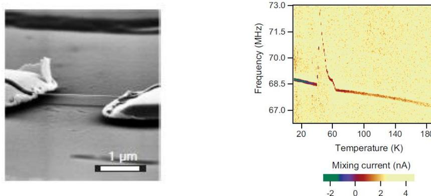
Fig. 1. (Left) Scanning electron microscope images of suspended NbSe<sub>3</sub> nanowires. (Right) Mixing current as a function of driving frequency and temperature. The CDW develops at 60 K and the sharp peak in resonant frequency at 42 K corresponds to a 12.8% change of the elastic modulus.
