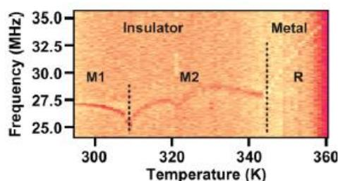
Fig. 2. The change in resonant frequency of a VO<sub>2</sub> resonator with temperature during the heating cycle from the insulator to the metallic phase.
