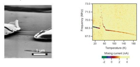
Fig. 1. (Left) Scanning electron microscope images of suspended NbSe<sub>3</sub> nanowires. (Right) Mixing current as a function of driving frequency and temperature. The CDW develops at 60 K and the sharp peak in resonant frequency at 42 K corresponds to a 12.8% change of the elastic modulus.
