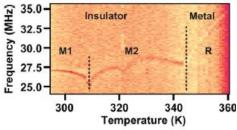
Fig. 2. The change in resonant frequency of a  $VO_2$  resonator with temperature during the heating cycle from the insulator to the metallic phase.
