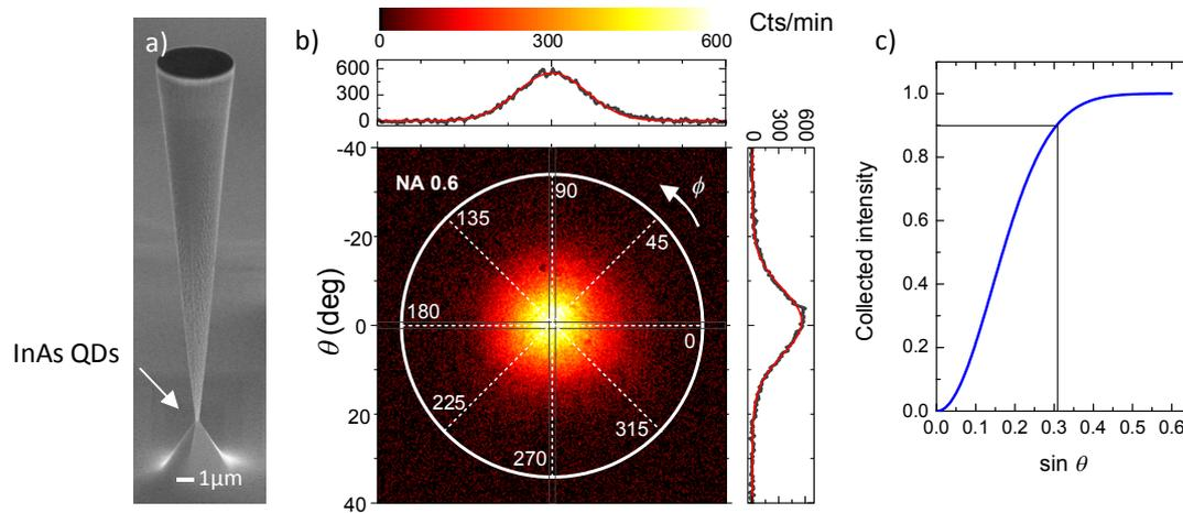
Figure 1: a) Scanning electron microscope image of the ‘giant’ photonic trumpet (tilted view). b) Giant trumpet’s far-field emission pattern with vertical and horizontal cut profiles shown in the top and the right panels. White circle corresponds to the maximum collection angle of the microscope objective (NA 0.6). c) Fraction of the collected beam intensity versus the collection NA.
