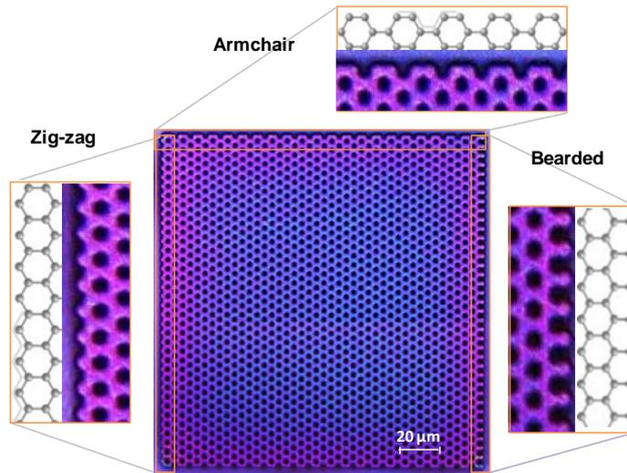
Figure 1 Optical microscope image of a polariton honeycomb lattice containing zig-zag, bearded and armchair edges.
