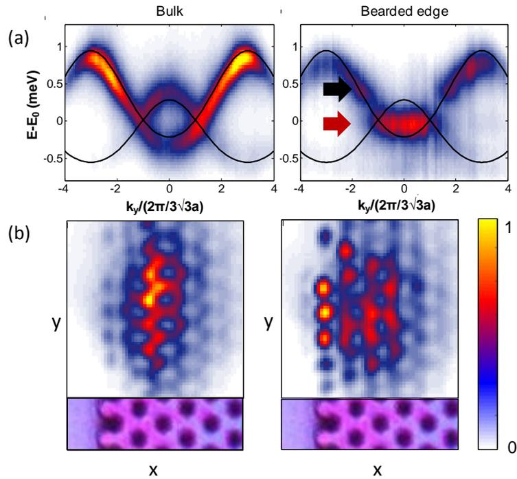
Figure 2 (a) Measured dispersion of the edge of the Brillouin zone probed in the bulk of the lattice and on the bearded edge, showing the flat dispersion characteristic of edge modes (marked with the red arrow). (b) Intensity of the real space emission measured at the energy of the bulk modes (marked with the black arrow in (a)), and at the energy of the edge state (marked with the red arrow in (b))
