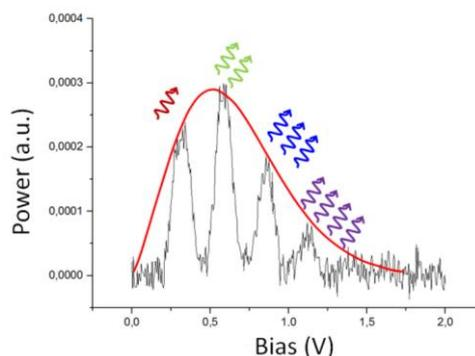
Figure 2: Dynamical coulomb blockage of Copper pair tunneling
