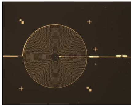
Figure 1: High impedance resonator in series with the Josephson junction
