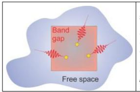
Scheme of how to probe the DOS in the band gap of a finite crystal by local probes. Quantum light emitters (yellow spheres) embedded in a finite photonic band gap crystal (square) experience the local density of states (LDOS) as the density of vacuum fluctuations (red wavelets). By averaging over many emitters throughout the crystal, we probe an average LDOS that represents the DOS of the finite crystal.
