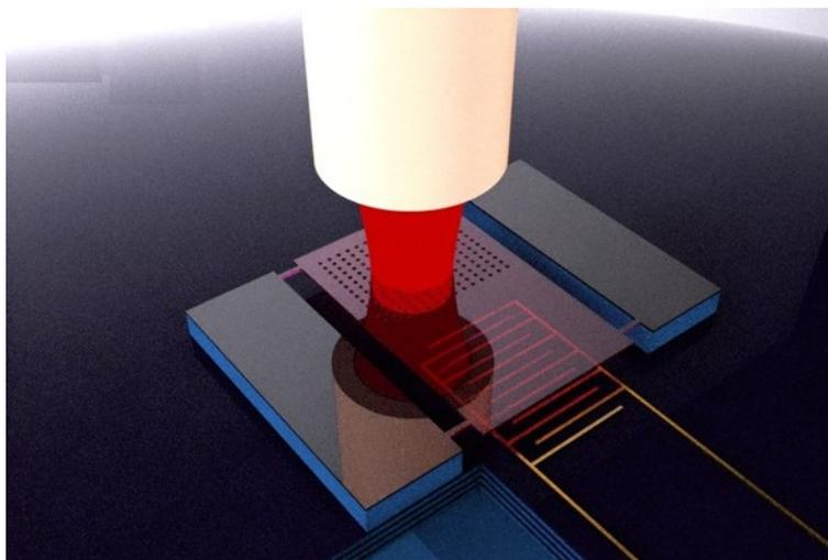
Example of a hybrid device coupling microwave and optical photons through their interaction with a suspended nanomembrane: its motion changes both the optical cavity length and the capacitance in the microwave circuit
